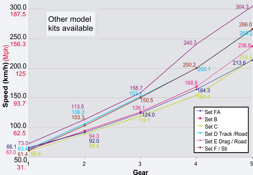
Speed in the gears at 7000rpm
